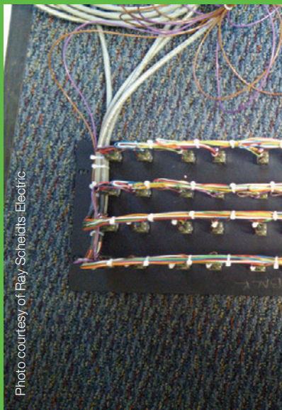
Image of the back of the Variac Heat Flux Control Panels built and installed by Ray Scheidts Electric.
